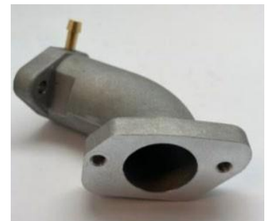
Intake Manifold 2023 Manifold 2023 PN: 138220034 Bore Diameter: 28.8mm Max
